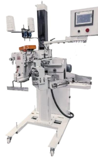
Automatic bag mouth folding and sewing machine is suitable for automatic folding and sewing of kraft paper bags or plastic woven bag mouths. Processes such as edge, stitching, trimming and thread cutting. Its air supply system realizes thread cutting. The height of the machine can be adjusted according to the size of the package. It can be combined with a conveyor to form an automatic production line, which is widely used in food, feed, chemical and other industries.
